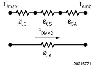
Once the maximum package power dissipation has been calculated using Equation 2, the maximum thermal resistance,  $\theta_{SA}$ , (heat sink to ambient) in  $^{\circ}\text{C}/\text{W}$  for a heat sink can be calculated. This calculation is made using Equation 3 which is derived by solving for  $\theta_{SA}$  from Equation 2.
